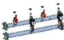
Collectors DN 80 to connect 2 or 3 boilers in the cascade system. Collector equipped with flange connections, isolation valves, non-return valves, reductions 1 1/2" x 1 1/4" and pumps Wilo Star RS 30/7, 12 UHR. These collectors allow assembly of cascades of 4, 5, 6, 7 or 8 boilers (see table "Elements of the cascades").
